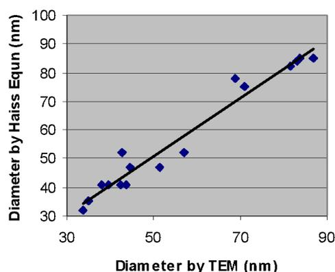
where  $d$  is the diameter of the SGNP,  $\lambda_{spr}$  is the wavelength at the peak of the surface plasmon resonance (SPR),  $\lambda_0 = 512$ ,  $L_1 = 6.53$ , and  $L_2 = 0.0216$ . Utilizing over 50 data points in his paper, Haiss finds an absolute error of 3%. Applying the equation to our gold nanoparticles determined by TEM, we find an error of 4%.
